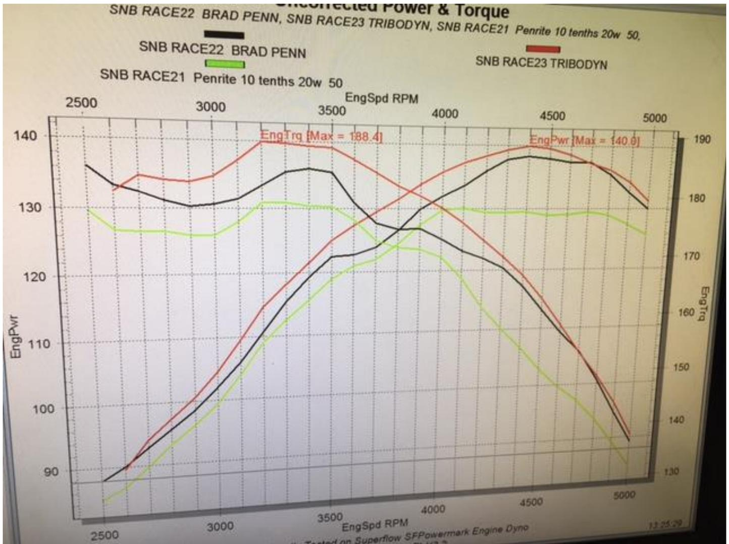
This Dyno test was on a SNB Race engine using 20W-50 oil. [www.snbracing.com.au](http://www.snbracing.com.au)
